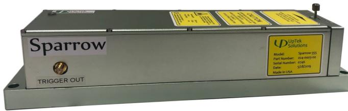
Sparrow is a diode pumped, water-free, passively Q-switched laser based on a microchip with multiple frequency conversion stages. Sparrow is optimized to produce  $TEM_{00}$ , low divergence, ~1 nanosecond pulses in a compact and robust package.
